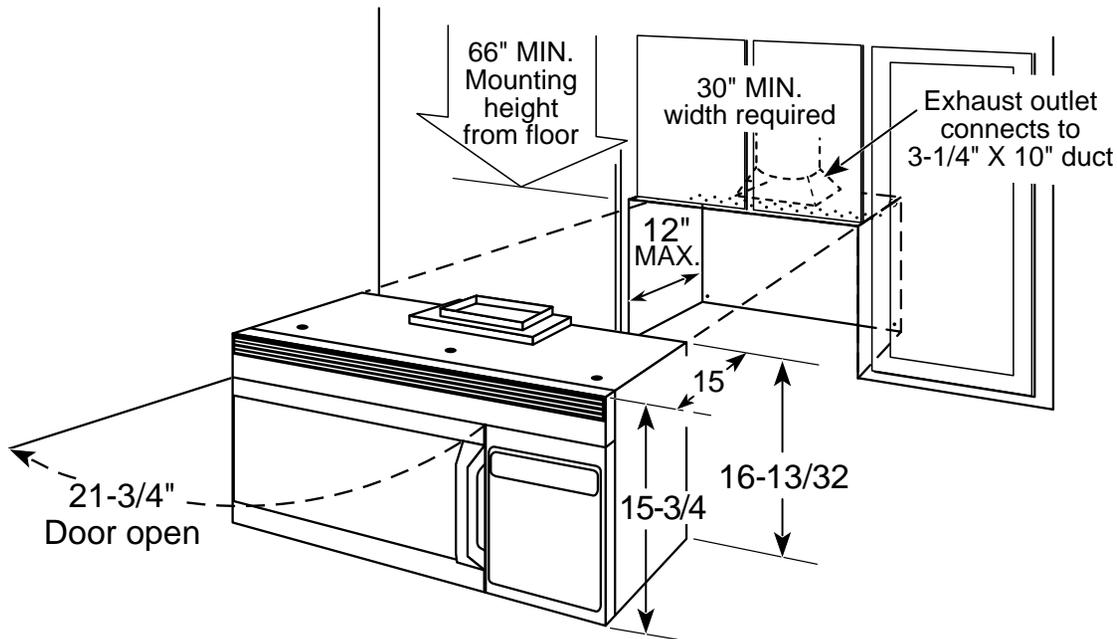
**Note:** Requires 120V grounded outlet. Electrical receptacle must be located in cabinet above Spacemaker microwave oven. No additional wiring, venting or cabinet rebuilding necessary in many cases. Complete detailed, easy-to-follow installation instructions and convenient full-size templates are packed with the Spacemaker microwave oven.
