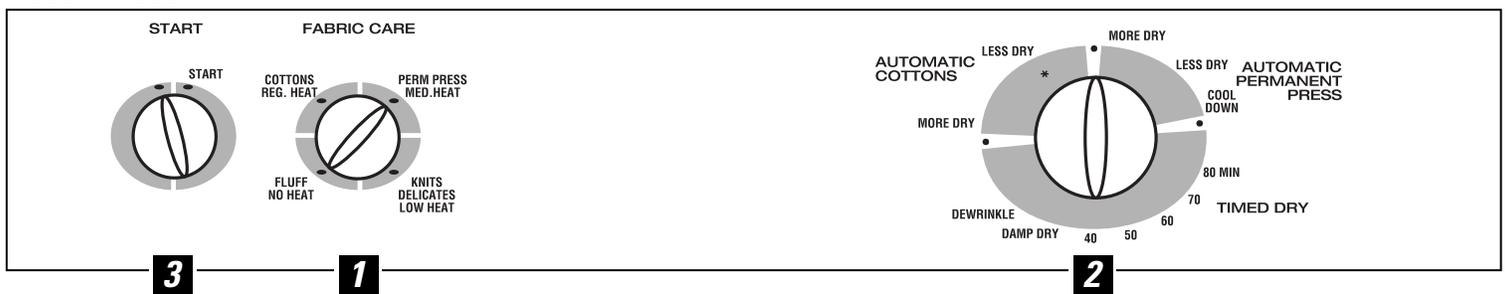
**NOTE:** Drying times will vary according to the type of heat used (Electric, Natural or LP gas), size of load, types of fabrics, wetness of clothes and condition of exhaust ducts.
