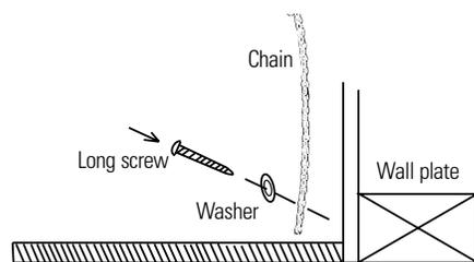
Make certain the screw is going into the wall plate at the base of the wall or one of the studs in the base of the wall.
