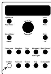
The vent fan removes steam and other vapors from surface cooking.
