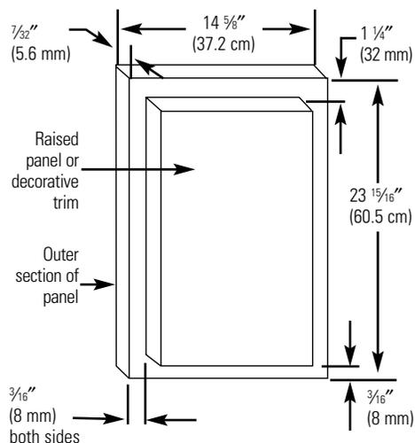
**Raised panel:** The outer section of the panel must be  $\frac{7}{32}$ " (5.6 mm) thick to fit into trim. Raised panel dimensions as shown above.
