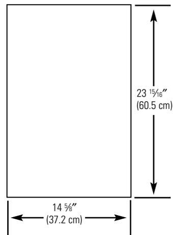
**Flat panel:** A  $\frac{7}{32}$ " (5.6 mm) thick panel is required. This is the same thickness as a standard  $\frac{1}{4}$ " plywood or paneling.
