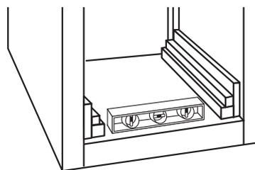
**8** Determine if you want the compactor frame or drawer front flush with the cabinet front.
