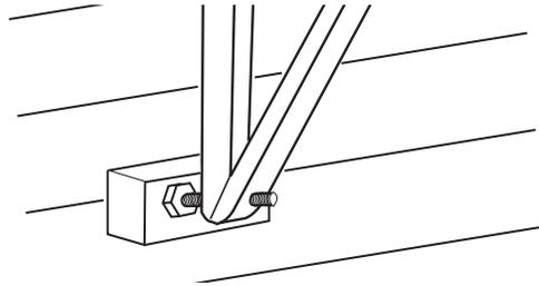
**NOTE:** Use a wood block between the leveling bolts and the wall if the wall is weak or if the weight of the air conditioner falls between the studs in the wall.
