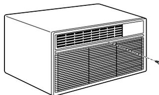
On models with a raise up inlet grille, lift it (see the Care and Cleaning section) and remove the screw behind it (if present) that holds the grille in place.
