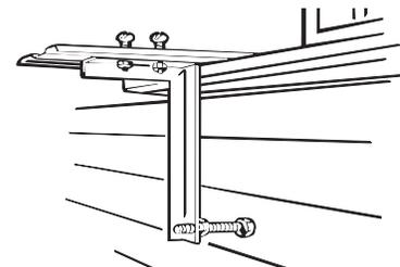
**NOTE:** DO NOT drill a hole in the bottom of the pan. The air conditioner is designed to operate with the bottom of the pan approximately half-full of water.
