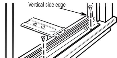
**NOTE:** To overcome interference of the support platform with the window track or storm window, securely attach a 2" wide shim strip to the window sill. This strip should be as long as the width of the support platform and flush with the back edge of the sill. The thickness of the strip should be controlled by the amount of interference.
