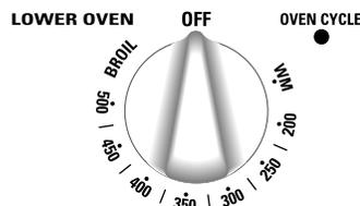
The **OVEN CYCLE** light glows until the oven reaches your selected temperature, then goes off and on with the oven element(s) during cooking.
