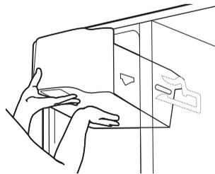
**2** Lift and pull forward again to remove the bin.
