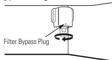
You must use the filter bypass plug when a replacement filter cartridge is not available. The dispenser and the icemaker will not operate without the filter or filter bypass plug.
