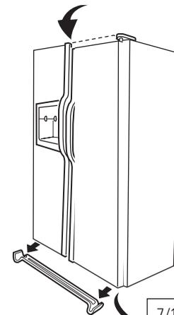
To remove the base grille, open the doors, remove the screw at each end of the base grille and then pull the grille straight out.
