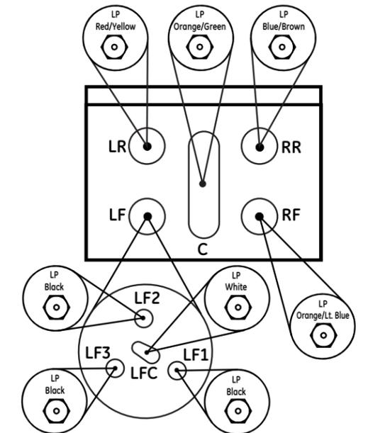
To prevent leakage, make sure the orifices are securely screwed into the gas supply tubes.
