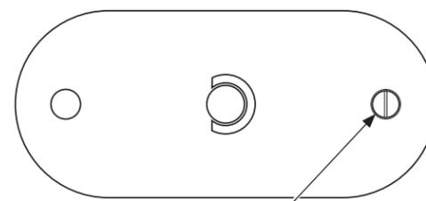
Right adjustment screw for extra-large burner
