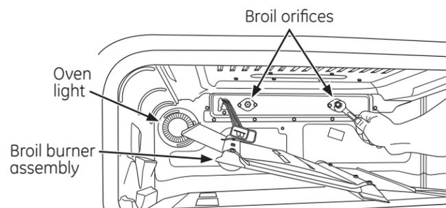
1. Remove the two 1/4" hex screws securing the broil burner and allow assembly to hang down free of the broil orifices.
