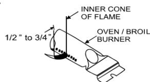
**NOTE:** If burner flames look like (A), further air shutter adjustment to the bake burner is required. Normal burner flames should look like (B) or (C), depending on the type of gas you use. With LP gas, some yellow tipping on the outer cones is normal.
