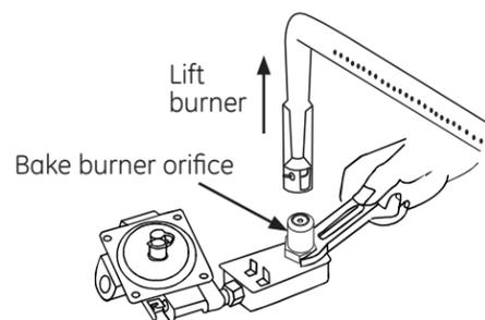
1. Remove oven racks, door, warming drawer and oven bottom. Remove the 1/4" hex screws securing the bake burner but don't remove burner from its location.
