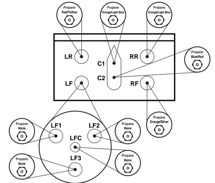
To prevent leakage, make sure the orifice spuds are securely screwed into the gas supply tubes.
