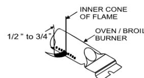
The combustion quality of the burner flames needs to be determined visually.
