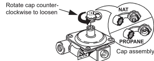
3. Turn the metal cap so the type of gas being converted to is displayed and replace the protective plastic cover.
