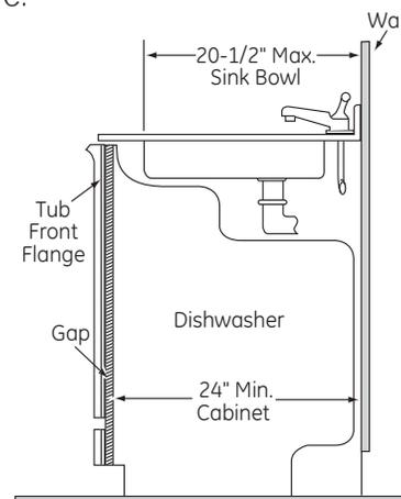
**Note:** A gap between the dishwasher tub front flange and the front of the base cabinet may result due to either the cabinet being less than 24" deep or the sink bowl not being installed to specifications.
