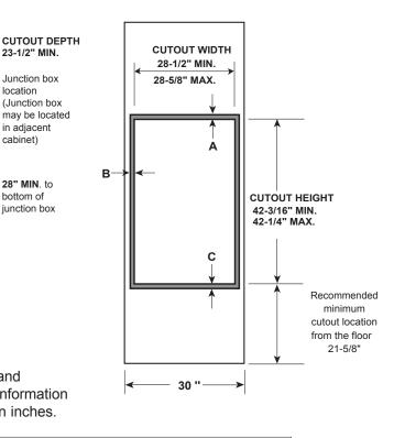
ATTENTION INSTALLER: All electric wall ovens must be hard-wired (direct-wired) nto an approved junction box. A plug and receptacle is NOT permitted on these products
