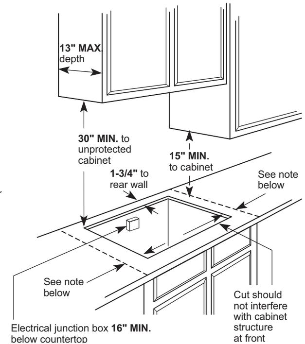
**NOTE:** This cooktop has been approved for 0" spacing to adjacent surfaces above the cooktop. However, a 6" minimum spacing to surfaces less than 15" above the cooktop is recommended to reduce the exposure to steam, grease spatter and heat.
