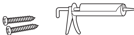
Wood screws and adhesive or other hardware for installing runners or shelf to support warmer drawer.
