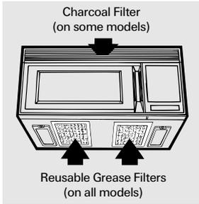
The vent fan has 2 metal reusable grease filters.
