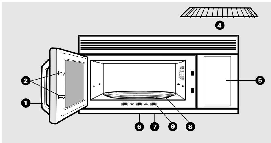
**1 Door Handle.** Pull to open the door. The door must be securely latched for the microwave to operate.
