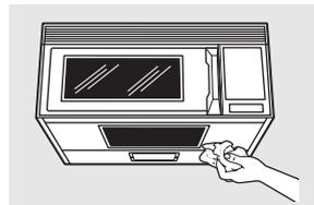
Clean off the grease and dust on the bottom often. Use a solution of warm water and detergent.
