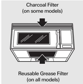
The vent fan has a metal reusable grease filter.
