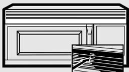
Remove 2 grille screws to remove the grille.
