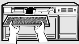
To install a new filter, remove plastic and other outer wrapping from the new filter.
