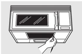
**To remove**, slide it to the side using the tab. Pull it down and out.
