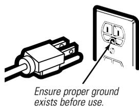
This appliance must be grounded. In the event of an electrical short circuit, grounding reduces the risk of electric shock by providing an escape wire for the electric current.
