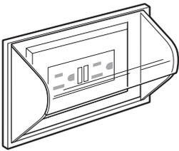
**Refrigerator MUST be plugged into a functioning GFCI circuit.** Test your circuit by plugging your refrigerator into the outlet and pressing the test button for that circuit, verifying that the unit turns off (the light will not work with the door open). Then press the Reset button and confirm that the light comes on with the door open. If you do not know if you have a GFCI circuit, contact a qualified electrician for assistance.
