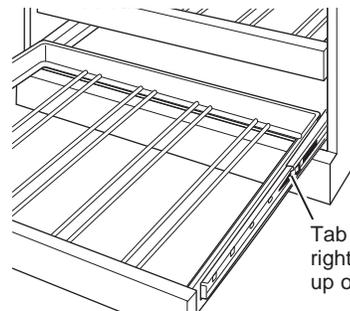
Tab (push tab down on right drawer guide, pull tab up on left drawer guide)
