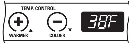
**To change the temperature setting,** press the WARMER or COLDER pads until you reach the desired set temperature. After 5 seconds, the display will return to the actual temperature.
