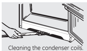
Cleaning the condenser coils.
