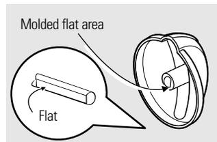
On some models, the knob stem is flat on one side (see illustration). Check the inside of the knob and find the molded flat area.
