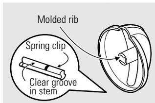
On some models, the knob stem has a groove in each side. The groove on one side has a spring clip. The other groove is clear (see illustration). Check the inside of the knob and find the molded rib.
