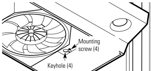
**NOTE:** DO NOT PUSH ON FAN BLADE. Pushing on the blade may cause it to interfere with other hood parts.
