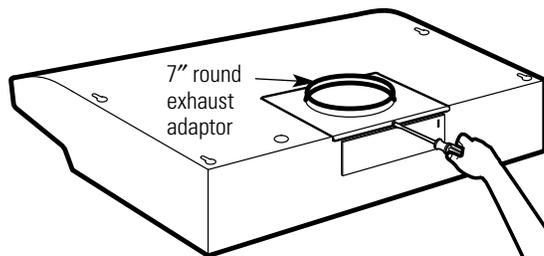
**NOTE:** The 7" round exhaust adaptor can be installed up to 1 inch on either side of the hood center to accommodate off-center ductwork. In extreme off-center installations, one end of the duct connector may need to be trimmed to clear the electrical cable clamp.
