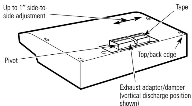
**NOTE:** The exhaust adaptor/damper can be installed up to 1 inch on either side of the hood center to accommodate off-center ductwork. In extreme off-center installations, one end of the duct connector may need to be trimmed to clear the electrical cable clamp.
