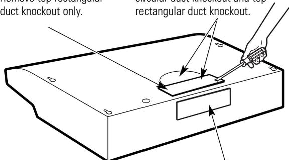
**3/4" x 10" Rectangular horizontal discharge.** Remove rear rectangular duct knockout only.
