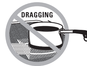
Do not slide cookware across the cooktop because it can scratch the glass—the glass is scratch-resistant, not scratch proof.
