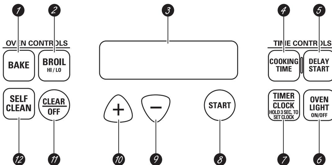
1. **BAKE:** Touch this pad to select the bake function. **Bake Light:** Flashes while in edit mode—you can change the oven temperature at this point. Glows when the oven is in bake mode.
