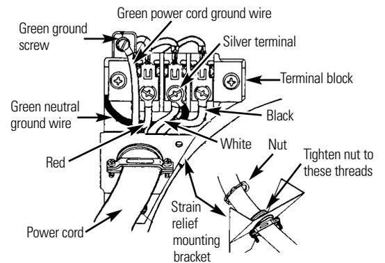
**⚠ WARNING:** Do not make a sharp bend or crimp wiring/conductor at the connections.
