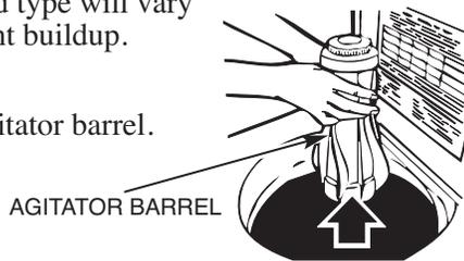
2. Wash or wipe the filter clean in the bottom of the agitator barrel. The filter is not removable.
