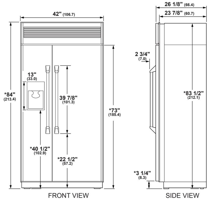
\* Shipping height. Use leveling legs and wheels for maximum 1" height adjustment from shipping height.
